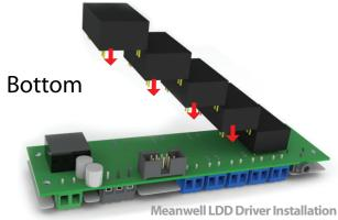
Modular LED Drivers provide the option for 300mA, 500mA, 700mA, or 1000mA of LED driving current.
